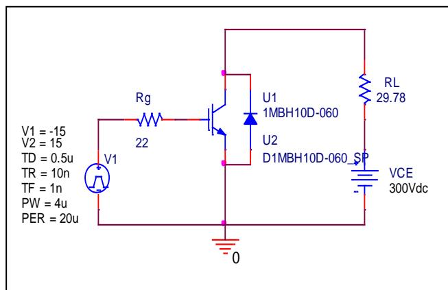
Test condition:  $I_C=10$  (A),  $V_{CC}=300$  (V)
