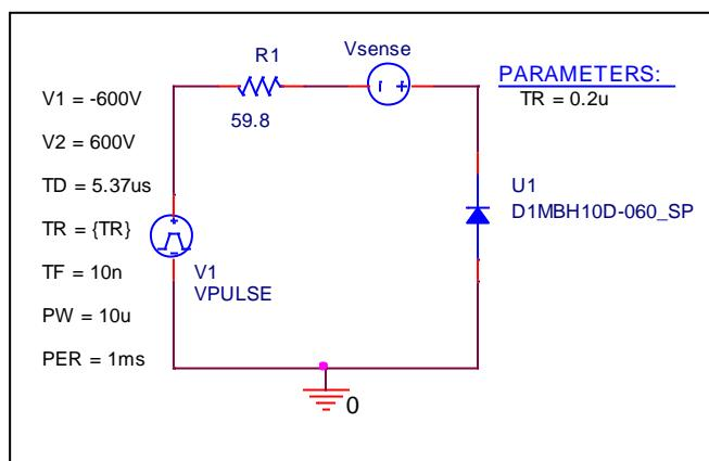
Test condition:  $V_{CC}=600$  (V),  $I_C=10$  (A),  $-dI/dt=100A/\mu sec$ .
