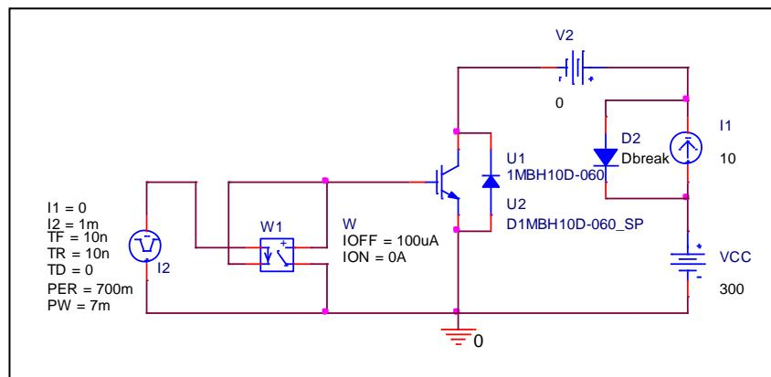
Test condition:  $V_{CC}=300$  (V),  $I_C=10$  (A),  $V_{GE}=15$  (V)
